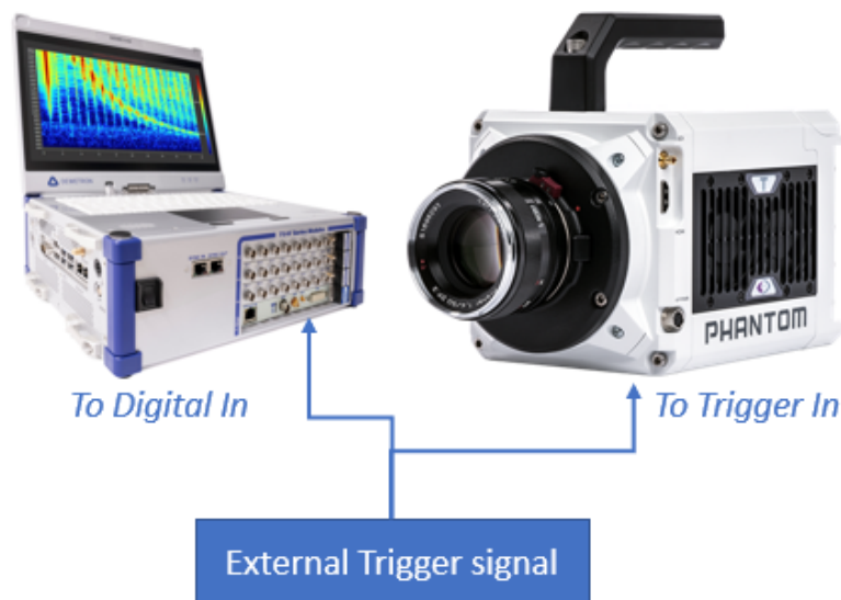
Fig. 7.163: Recording start of DAQ system and camera triggered by external signal
