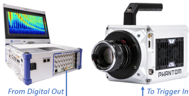
Fig. 7.165: Recording start of camera triggered by DAQ system
