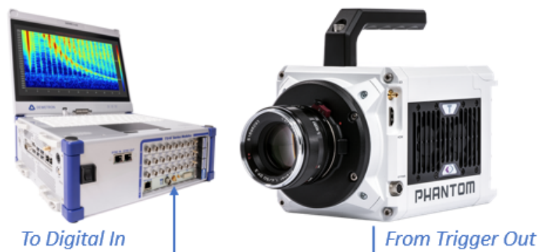
Fig. 7.164: Recording start of DAQ system triggered by camera
